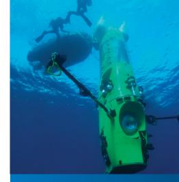
Deepsea Challenger is a 24 ft deepdiving submersible designed to reach the deepest-known point on Earth. The vehicle operates in a vertical attitude, and carries ballast weight that allows it to sink to the bottom, and when released, rise to the surface.
